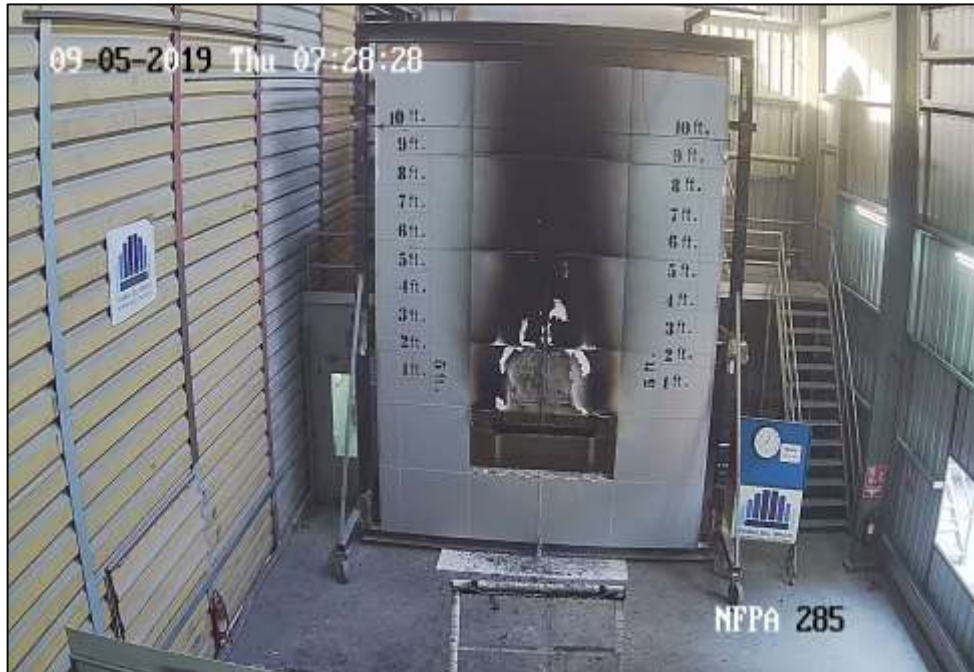
Picture 13: The specimen at the end of the observation period and end of the NFPA 285 test.
