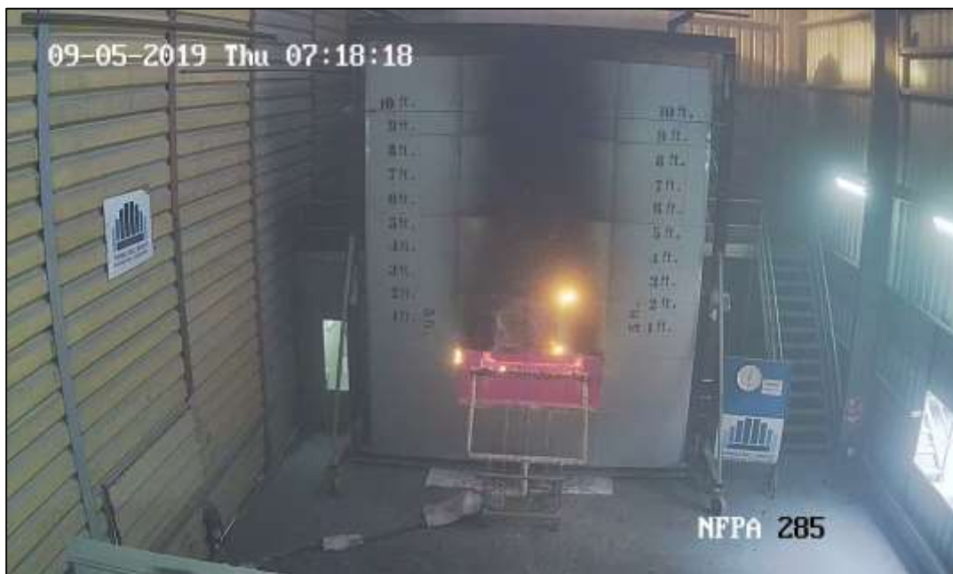
Picture 11: The specimen immediately after the gas was shut off, starting the observation period.
